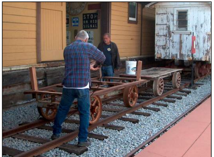
In 2015 Tom Cooper (back to camera) and Ted Van Klaveren resist the urge to joyride and instead prepare one of the Museum’s narrow-gauge push-cars to hold a load of timber pilings, as it would have on the Pacific Coast Railway wharf at Port San Luis. The nearer car was owned by Union Oil, the other car by PCRY. Photo by Glen Matteson.
