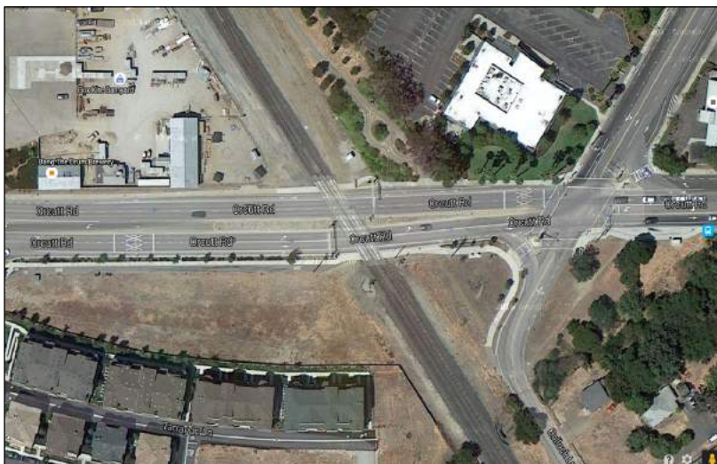
This close-in Google Satellite view shows townhouses curving away from Orcutt Road, and Bullock Lane angling to align with Laurel Lane, so that someday this grade crossing may more easily become part of history if a bridge is built.
