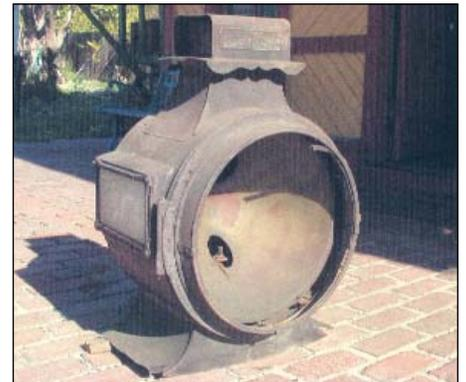
*The headlight above is a carbide light made by the U.S. Headlight Company of Buffalo, N.Y. Patented November 28, 1887. The red light is a kerosene light made by the Roesch Lamp Company, of San Francisco, California.*
